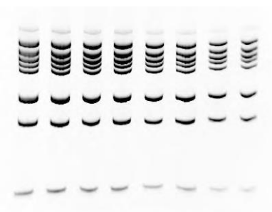
EtBr stained acrylamide gel excited through MD-25 UV transilluminator
